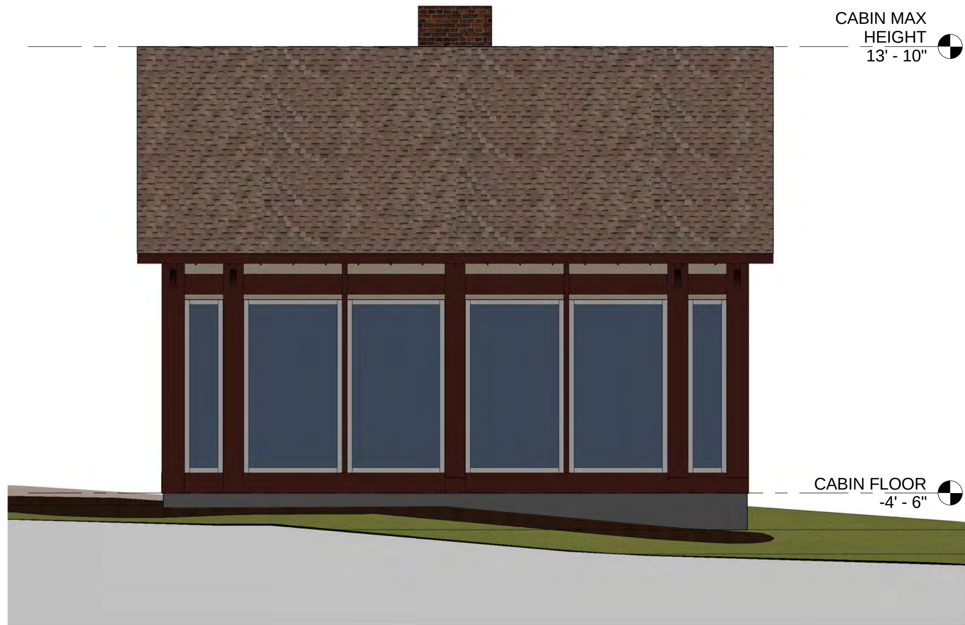
2 CABIN NORTH ELEVATION A270 1/4" = 1'-0"
