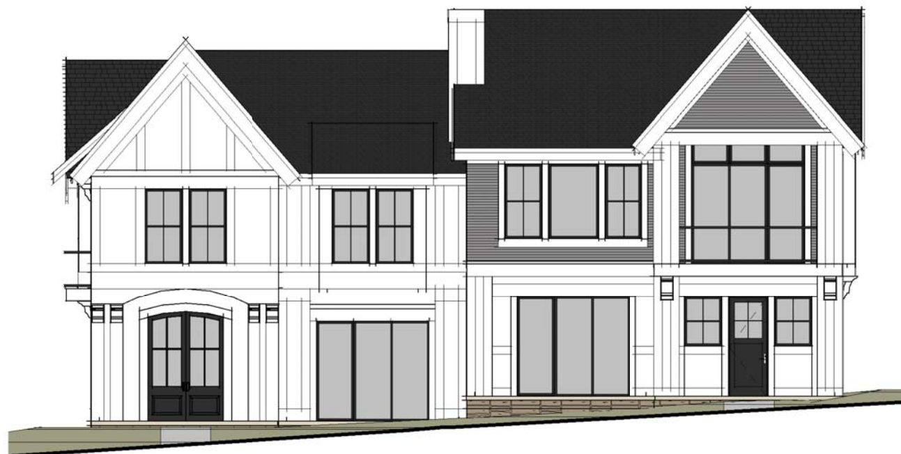
EAST ELEVATION BLDG. B UNITS 4 & 5 SCALE: 3/32" = 1'-0"
