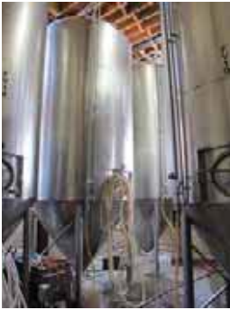
Stainless Steel Tanks for Fermentation
