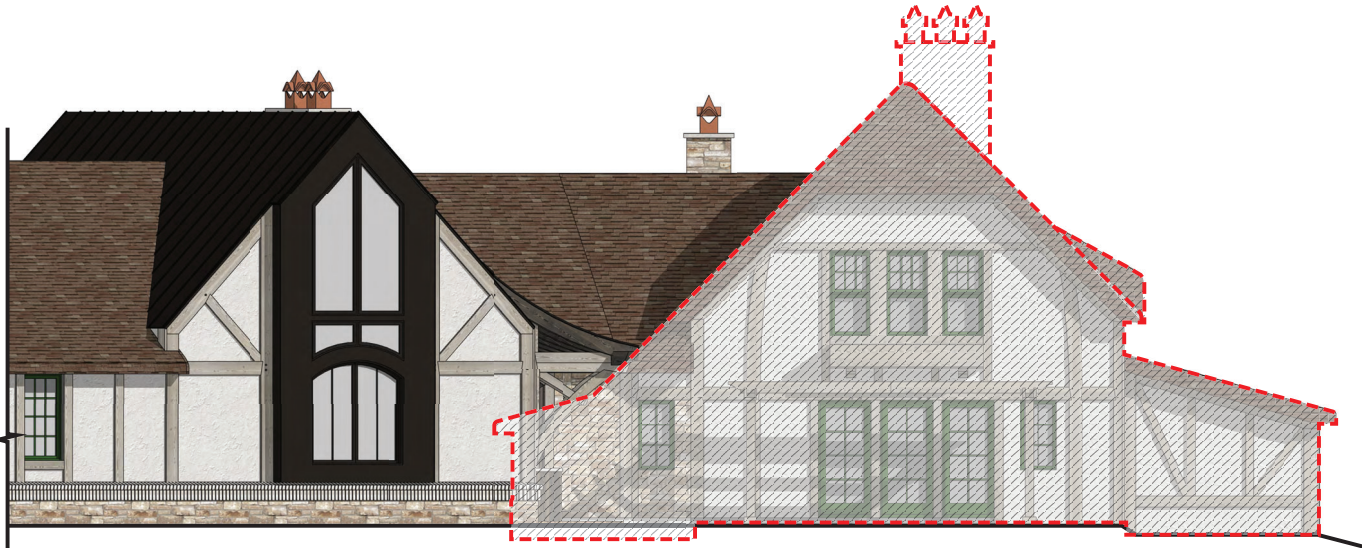
2 1.3 EXISTING HOUSE SHOWN OVER PROPOSED - STREET SIDE ELEVATION SCALE: 1/4"=1'-0"
