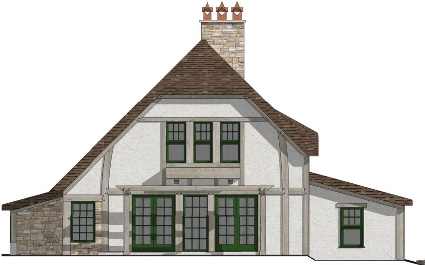
1 1.3 EXISTING HOUSE - STREET SIDE ELEVATION SCALE: 1/4"=1'-0"
