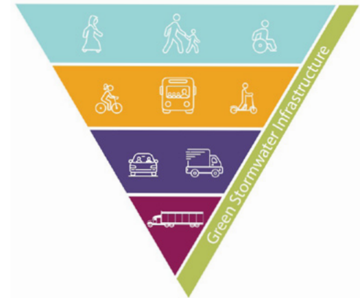
Complete streets’ hierarchy places pedestrians at the top and integrates green stormwater infrastructure throughout (Image source: City of Minneapolis)
