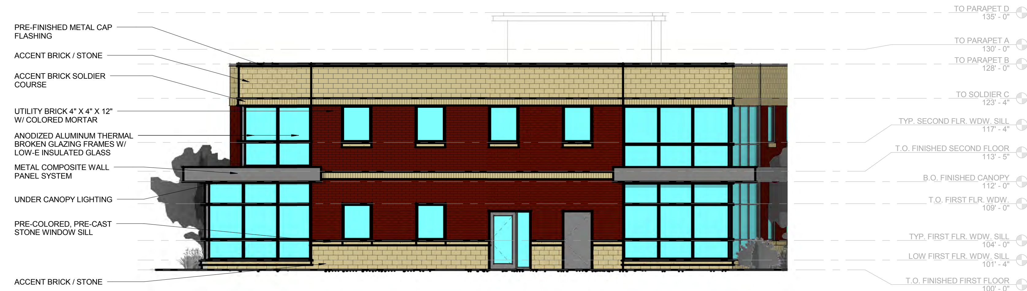
4 EXTERIOR ELEVATION WEST PZ-2 1/8" = 1'-0"
