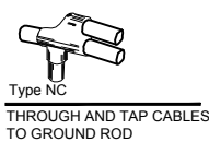
1 EXOTHERMIC WELD DETAILS EXOTHERMIC AND HARGER ULTRAWELD OR APPROVED EQUAL
